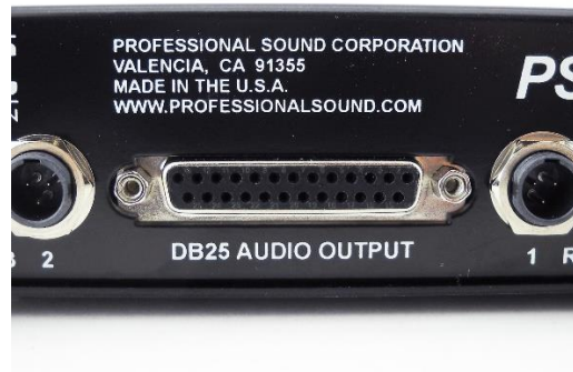
All Audio Outputs on Multi-Pin Snake Tascam™ Wiring Standard
