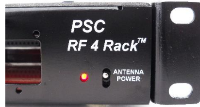
Remote Antenna Power Switch
