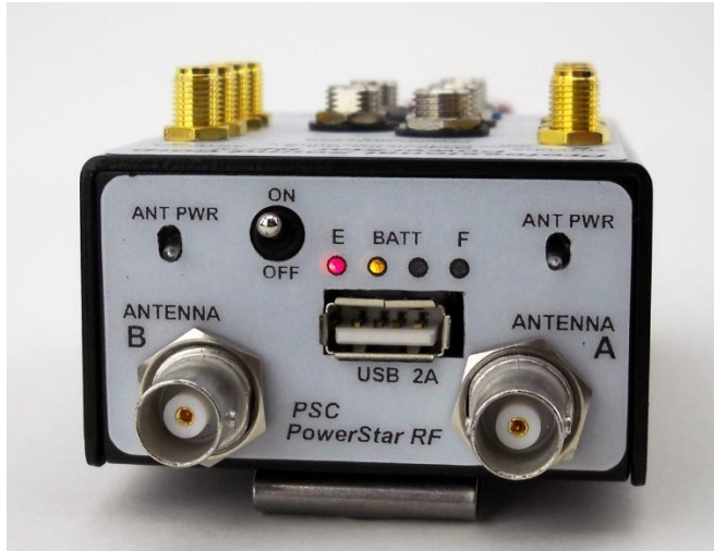
2 of 4 LEDs lighted, indicating 50% charged battery
