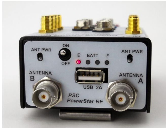
RED LED only lighted, indicating less than 25% battery charge
