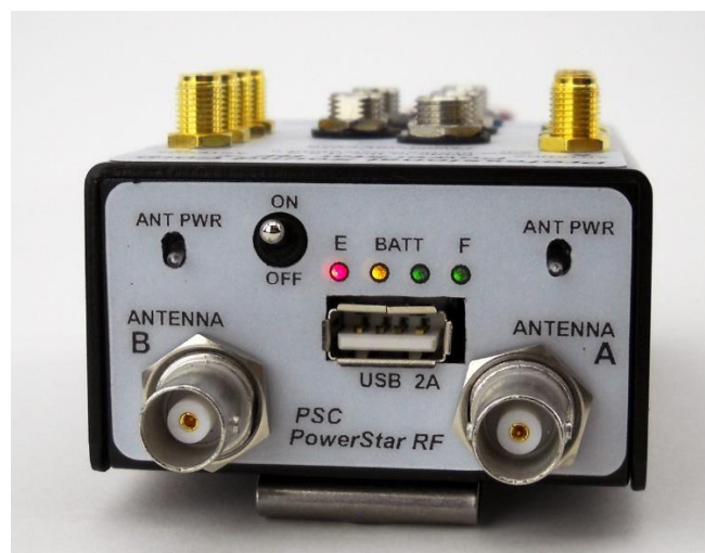
All LEDs lighted, indicating a full battery
