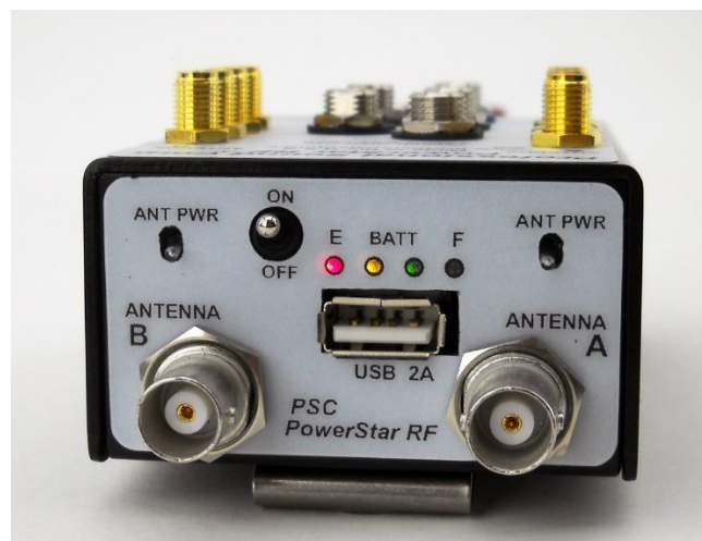
3 of 4 LEDs lighted, indicating 75% charged battery
