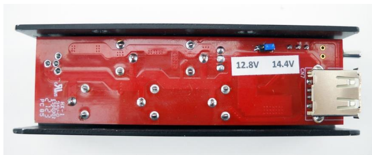
Blue “Battery Type” Jumper set for use with 14.4 volt battery
