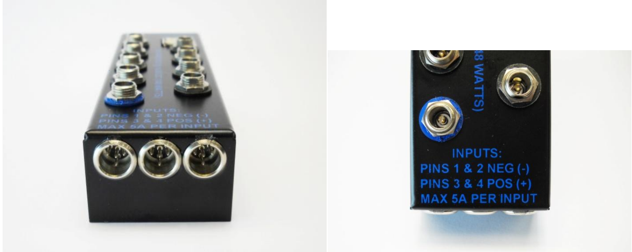
THREE (3) POWER INPUT CONNECTIONS ON TB4M CONNECTORS
