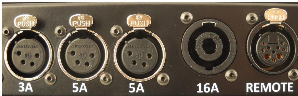
SpeakOn Connector used to supply heavy current devices
