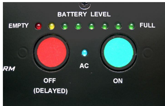
Battery “Fuel Gauge”
