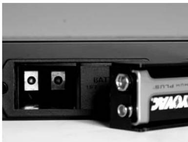
Install two, fresh 9V alkaline batteries noting the correct polarity.
