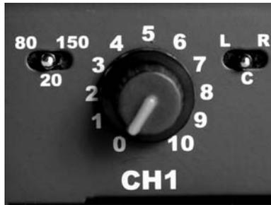
For basic operation, set all pan switches to the center (C) position.
