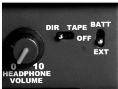
Set the power switch to the internal battery by moving it upward towards the "BATT" marking.
