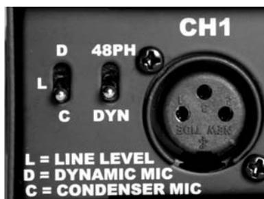
Select the appropriate input level by selecting "D", "L" or "C" on the toggle switch located next to each input XLR connector. Select "D" for use with Dynamic microphones (non-powered microphones). Select "L" for use with line level sources such as the line outputs from CD players. Select "C" for use with condenser microphones (48PH powered microphones).
