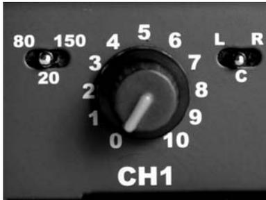
Slowly open the channel fader pot unit you reach the desired operating level for each input. Always try to operate the mixer so that the audio signal displayed on the meters is just peaking to the “0” indicator (first amber LED).
