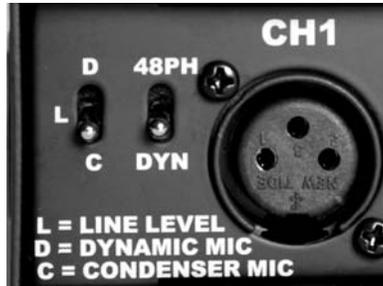
Select “48PH” microphone power or “DYN” by selecting the switch located next to each input XLR connector. Only select “48PH” when using microphones designed to operate from 48PH or 9-52PH or 9-52 simplex power. For all other uses, select “DYN”.
