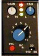
Just to the right of each gain control are the AlphaMix **retracting pan pots**. These are equipped with center detents to confirm mid placement in the summing output bus. As with any pan pots; the signal may be positioned as desired within the stereo field. Once placement has been determined the pots can be recessed to keep the front panel free from obstruction while mixing.
