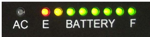
Unit Not Plugged Into AC Power
