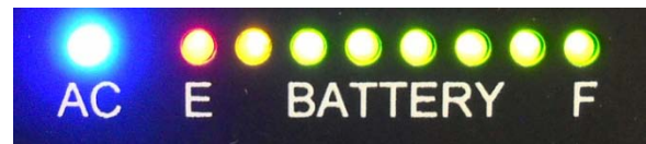
Unit Plugged Into AC Power
