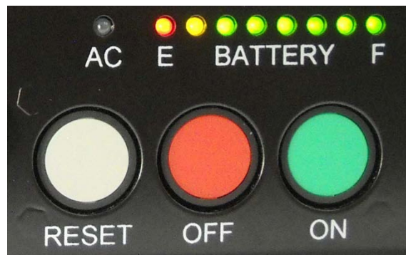
“RESET” switch located under the AC LED
