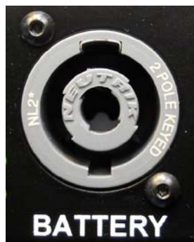
SpeakOn Connector used to external battery connection
