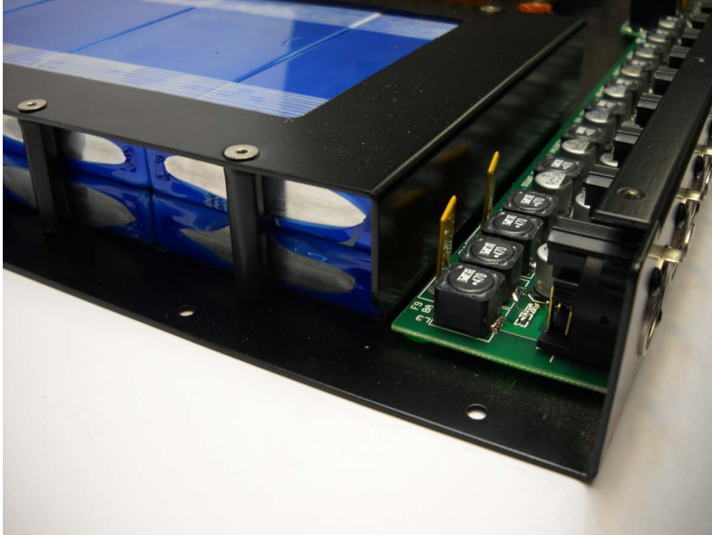
PSC Quiet Power tm Filters partially shown behind output XLRs.
