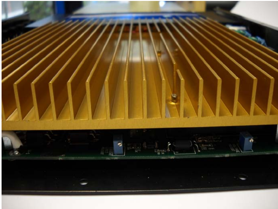
Close up view of the custom made, gold anodized, PSC aluminum heat sink extrusion
