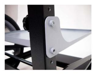
11. Gently push the thumb screws through the holes in the upright rails ensuring that they line up with the threaded inserts in the shelf ears and just start the threads. DO NOT COMPLETELY TIGHTEN THUMB SCREW AT THIS TIME! FINAL TIGHTENING WILL BE DONE AFTER THE CART IS COMPLETLEY ASSEMBLED!
