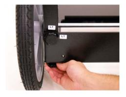
7. Locate the two (2) boom Cups with the two (2) of the ¼-20 SHORT Thumb Screws. Install the two boom cups by inserting the thumb screws though the boom cups and threading them into the threaded inserts in the rear of the cart base as shown in the photo below:
