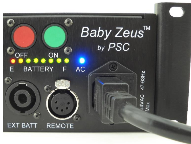
BLUE LED indicating AC power is connected
