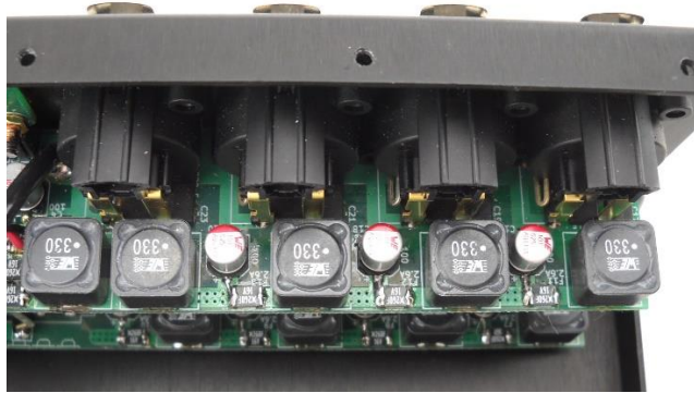
PSC Quiet Power™ Filters partially shown behind output XLRs.
