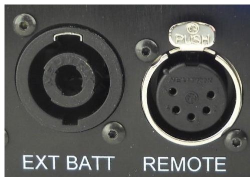
SpeakOn Connector used to external battery connection
